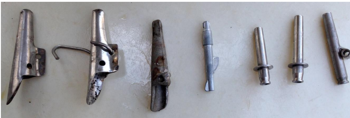
Figure 30. Assortment of spiles used during 2016.
