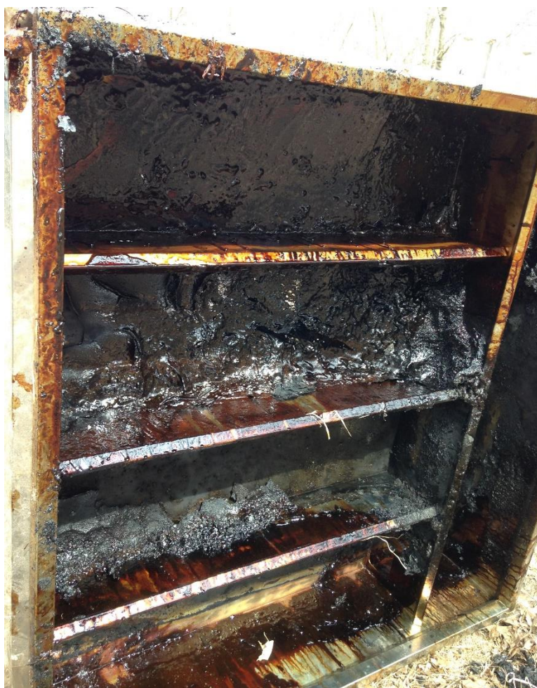
Figure 31. Burned syrup pan. Top image shows warping on the bottom of the pan. The lower image shows the caramelization and burning of the syrup in the pan.
