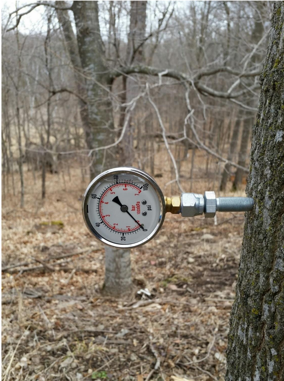
Figure 5. Gauge used to measure maple stem pressure during the sap flow season. Pressures can reach 30 psi and higher when the sap is flowing. Image by Br. Walter Kieffer, OSB.
