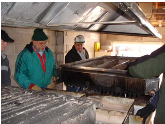
Figure 4. Bill Mock (green jacket) and Br Walter setting the pans in the evaporator.
