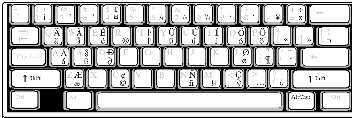
Figure A-1 The US International keyboard layout lets you type special characters not available on the US English keyboard layout.
