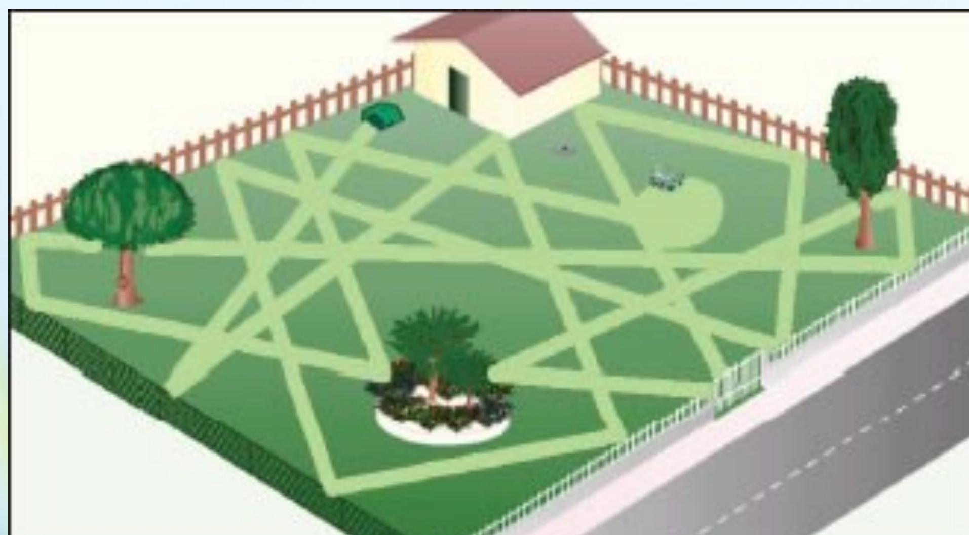
Fig 2. Random mow path created by robotic lawnmower (Lawnbotts.com)
