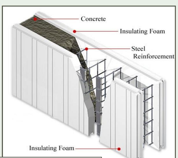
Insulated concrete forms, or ICFs, are expanded polystyrene (EPS) insulation sheets or blocks used as forms for poured concrete walls, then left in place to insulate the wall. They excel in energy efficiency and durability, but they are expensive and there are some air quality concerns with the EPS insulation used to make most ICFs. Photo: http://nickbugbee.files.wordpress.com/2011/01/icf-walls.jpg
